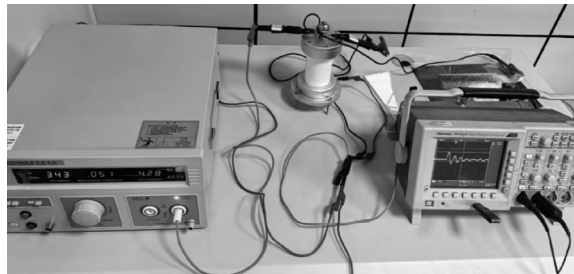
图12 自愈特性试验线路图 Fig. 12 Self-healing characteristic test circuit diagram
